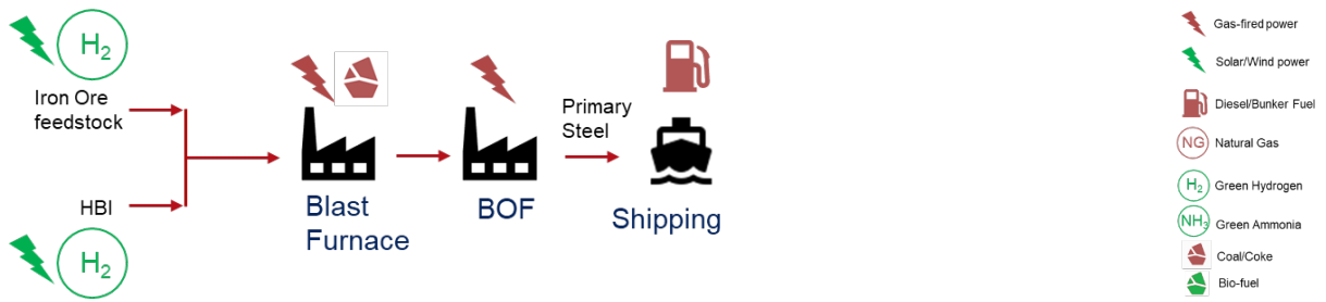
Figure 6.9 Use of green iron in the BF and BOF
